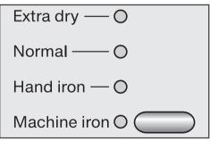
Press the drying level button repeatedly until the indicator for the drying level you want lights up.
